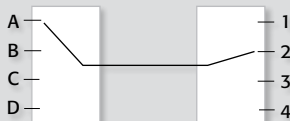
Figure 3. For improved flexibility, a series of switches can be arranged in a blocking matrix to connect multiple instruments to multiple DUTs.
