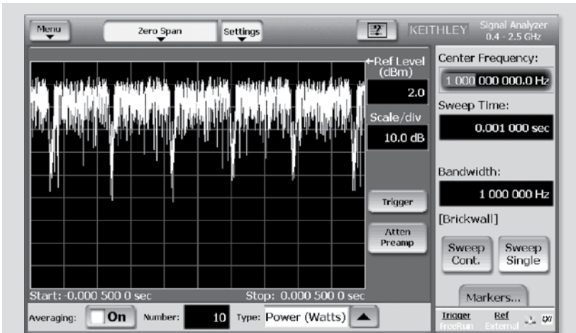
Figure 3a. 802.11A 64QAM signal with 0% compression in zero span
